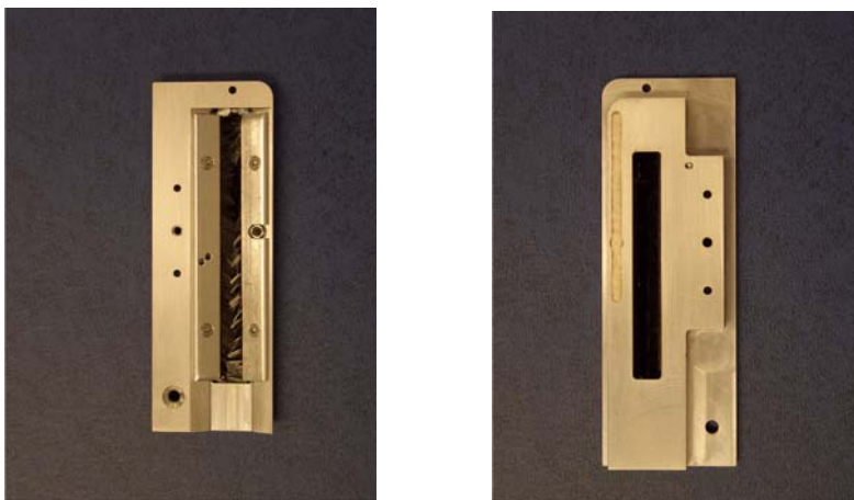
Figure 1 Modified top plate. Top view showing the brushes (left) and bottom view showing the wick (right). Your modified top plate may look slightly different, but it must have the brushes and wick to function effectively.
