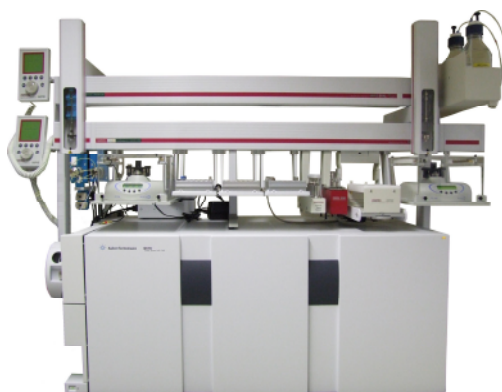
Figure 2. MPS 3 XL Prepstation configured for online QuEChERS.
