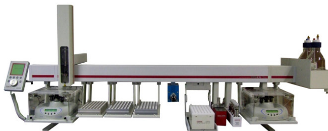
Figure 1. MPS 3 configured for offline QuEChERS automation.
