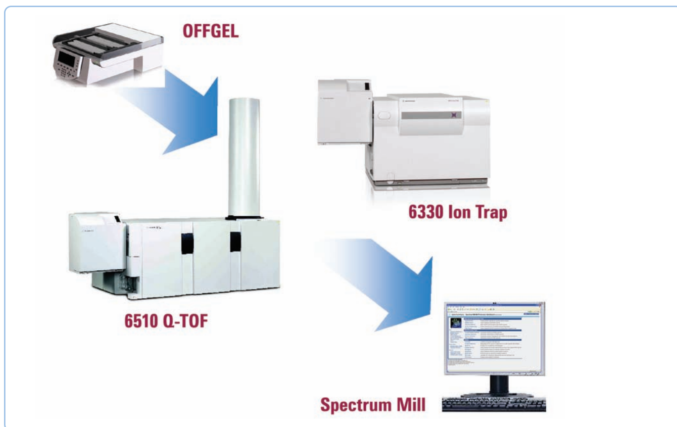
Figure 1. The experimental workflow consisting of a 3100 OFFGEL Fractionator, a 1200 HPLC-Chip/6510 Q-TOF LC/MS, and Spectrum Mill software for data analysis. As part of this study, the performance of the Q-TOF was compared with the 6330 Ion Trap mass spectrometer.
